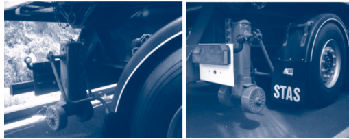
Figure 8.6.1.a. – Landing legs at the back
