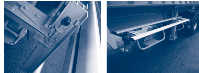
Figure 10.3.b. – Pull out safety pin and folding side guard upwards
