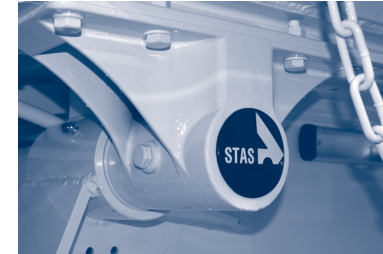
Figure 3.a. – Bolts for tipping shaft locking
