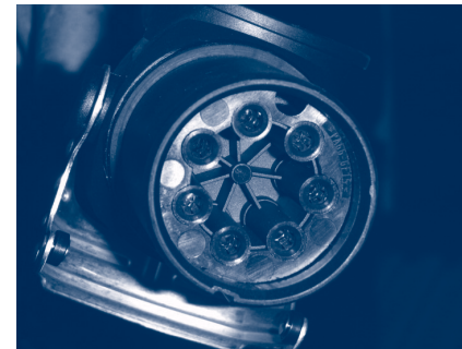
Figure 3.3.b. – 7-pin socket (left) and 5-pin socket (right)
