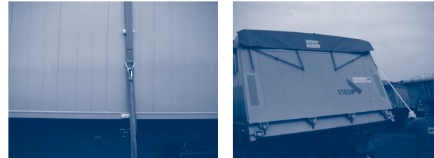
Figure 7.3.2.a. – Fastening pull back cord and loosening of roof sheet
