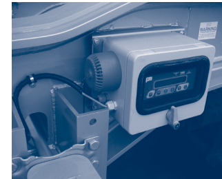
Figure 8.5.1.a. – Weighing equipment measuring unit
