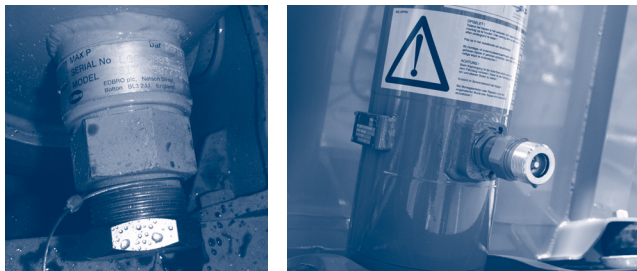
Figure 4.1.a. – Cylinder type plate + maximum cylinder pressure pictogram
