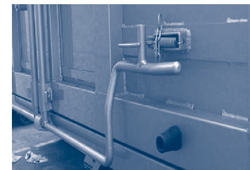
Figure 6.1.2.a. – Closing safety system
