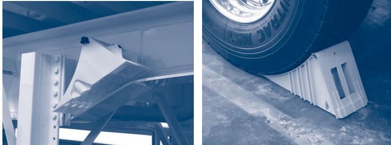
Figure 5.3.a. – Wheel chock in holder (left) and in place (right)
