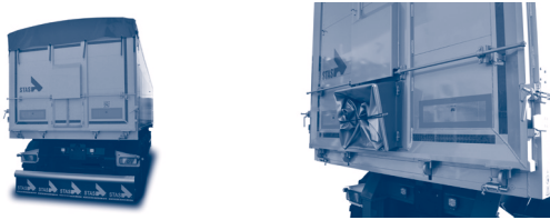
Figure 8.2.1.c. – Operation and locking of the grain hatch, type with rack and pinion
