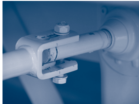
Figure 2.2.1.b. – Landing leg handle "steel type" pulled out
