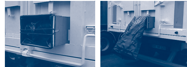
Figure 8.2.1.b. – Door with grain hatch with dust sleeve
