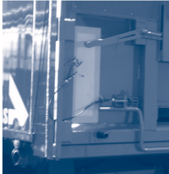
Figure 6.1.2.b. – Optional: opening barn door from the side of the trailer
