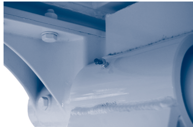
Figure 6.c. – Lubricate tipper turning points
