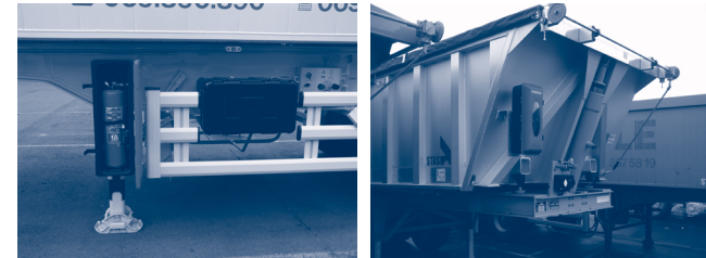
Figure 8.7.a. – Location of fire extinguisher on the tipper
