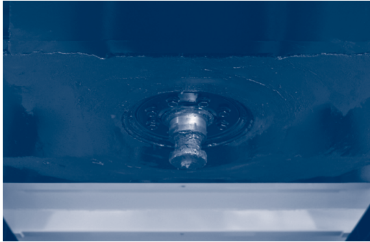
Figure 1.a. – Fifth wheel rubbing plate with kingpin
