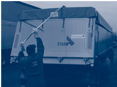
Figure 7.3.1.a. – "Dawnbarn" type roof sheeting system
