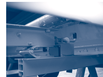
Figure 10.3.c. – Side guards folded up and secured
