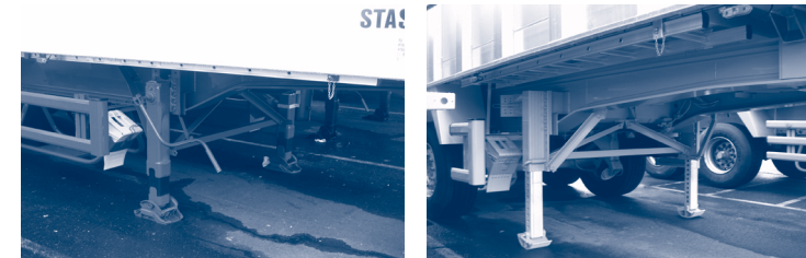
Figure 2.1.a. – “Steel type” (left) and (right) “aluminium type with two landing legs”
